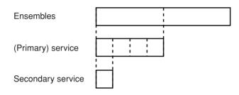
The unit can receive ensembles in frequency band III (174.928 – 239.200 MHz) and store their services in each ensemble. The number of ensemble you receive varies depending on your location. Band III is divided into 41 channels identified as 5A to 13F. Each channel can contain one ensemble. Channels allocated to the United Kingdom are in the range 11B to 12D.
