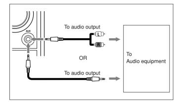
When the audio equipment has pin jacks for audio output: Be sure that the pin plugs of the audio cords are colored—white plugs and jacks are for left audio signals, and red ones for right audio signals.
