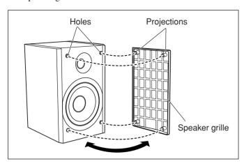
To remove the speaker grille, insert your fingers around the projection at the top of the speaker grille, then pull gently towards you while holding the side.
